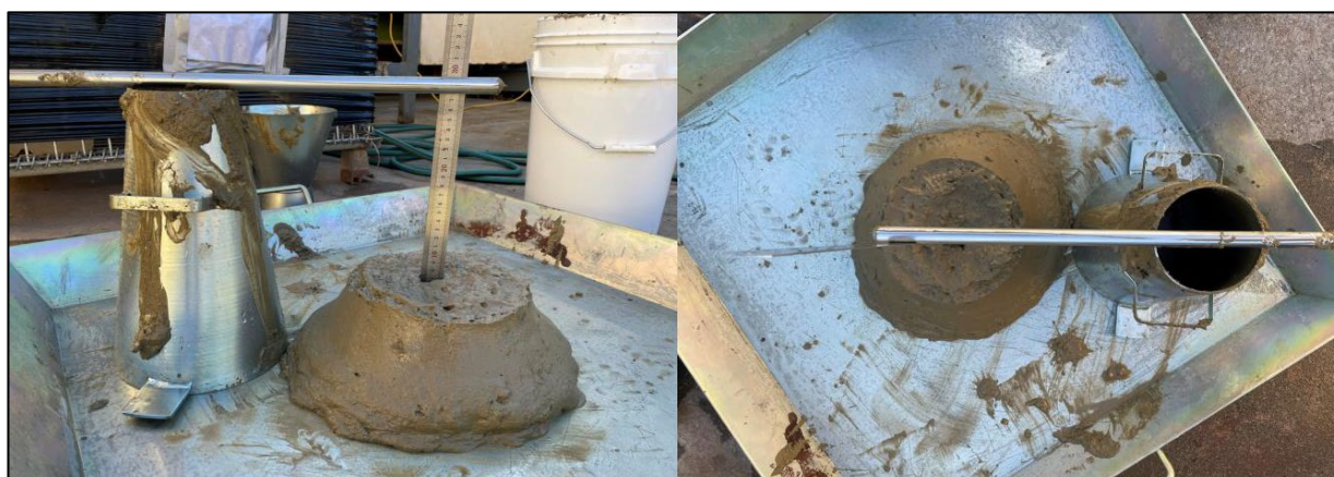
Figure 6: Slump Test (200mm) picture of 4% GP cement
